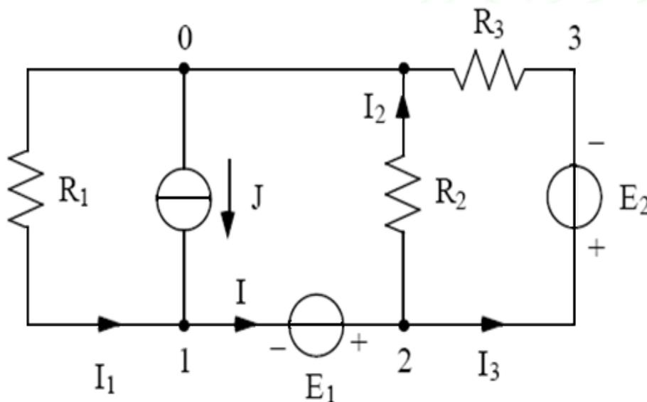
$$E_1 = 12 \text{ V}, E_2 = 6 \text{ V}, J = 5 \text{ A}, R_1 = 15 \text{ } \Omega, R_2 = 3 \text{ } \Omega, R_3 = 6 \text{ } \Omega.$$
