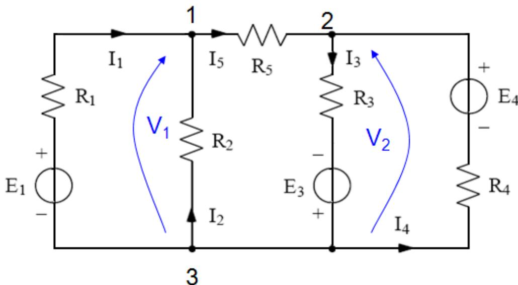
$$E_1 = 10 \text{ V}, E_3 = 70 \text{ V}, E_4 = -20 \text{ V}, R_1 = 10 \text{ } \Omega, R_2 = 5 \text{ } \Omega, R_3 = 2 \text{ } \Omega, R_4 = 4 \text{ } \Omega, R_5 = 1 \text{ } \Omega.$$
